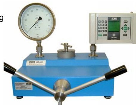
BT400-OX with Calibrator LPC 300 and test item
